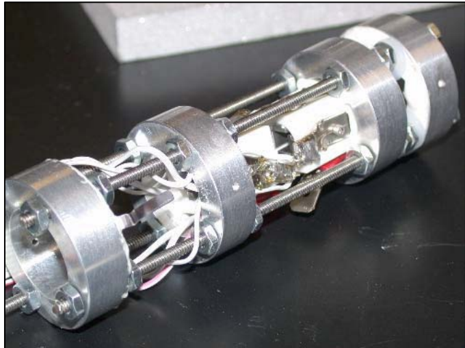
Figure 3. JPL RFMS prototype of August 2004; the unit is 4 inches long.
