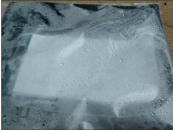
Figure 3. Salt water contained under the white ePTFE material is vaporized by solar energy and then condenses on the clear collection bag surface.
