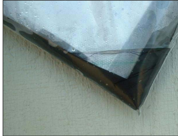
Figure 4. Approximately 25 milliliters of fresh water was produced by the EPWD after 5 hours of exposure to sunlight.
